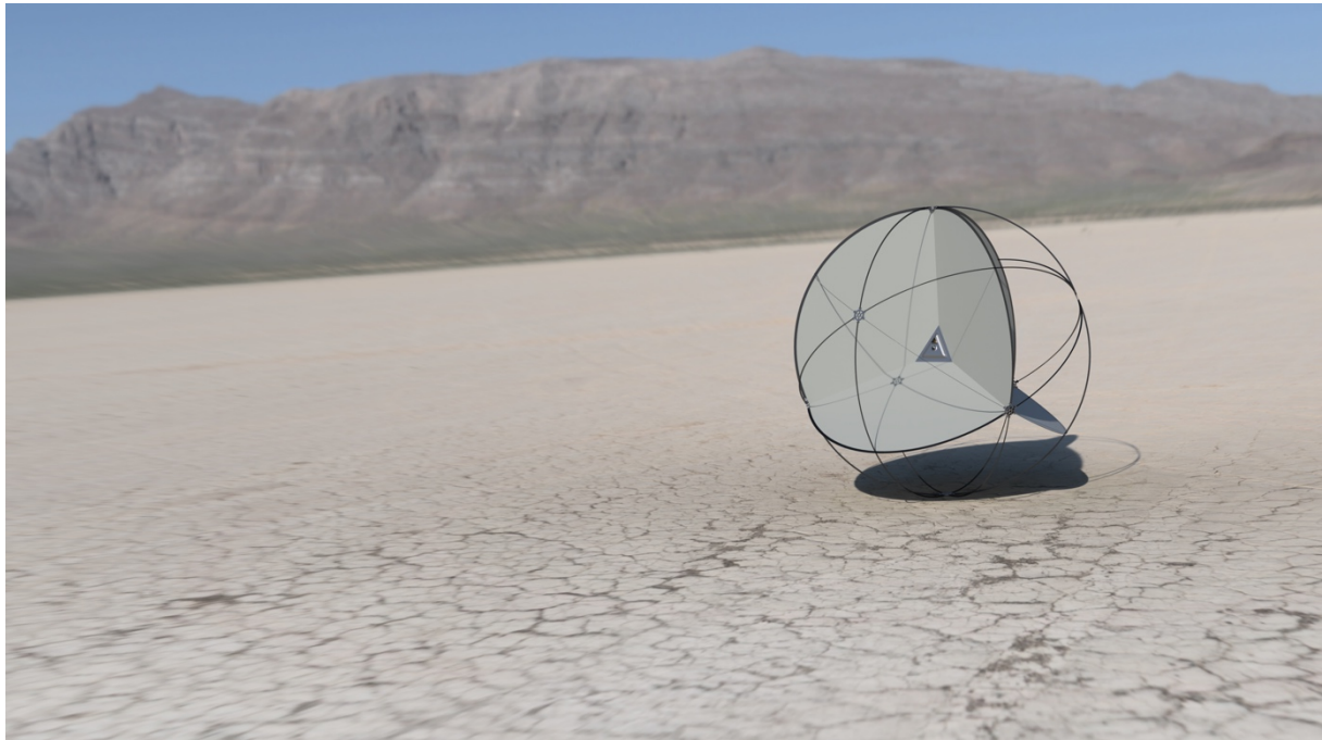
Figure 3: Rendering of the Tumbleweed Rover, with sails for harvesting Martian winds and the computing unit in the center.
