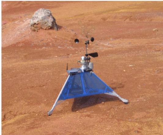
**Figure 1. HUNVEYOR-4 during a Martian analog terrestrial field study**
