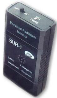
Figure 6. The personal radiation detector
