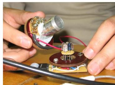
Figure 5. The student made LED spectrometer
