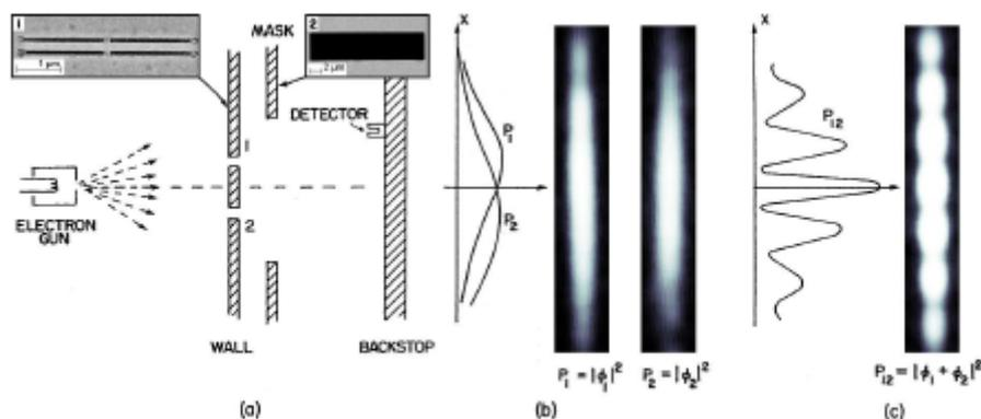
Fig. 1. The double slit experiment (from Ref. 2).
