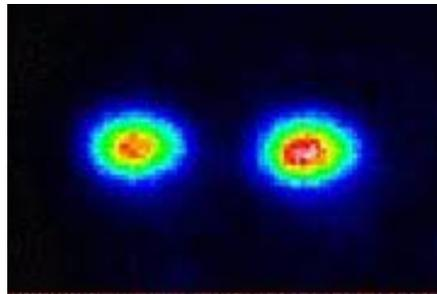
**Fig. 7. Two trapped ions.**
